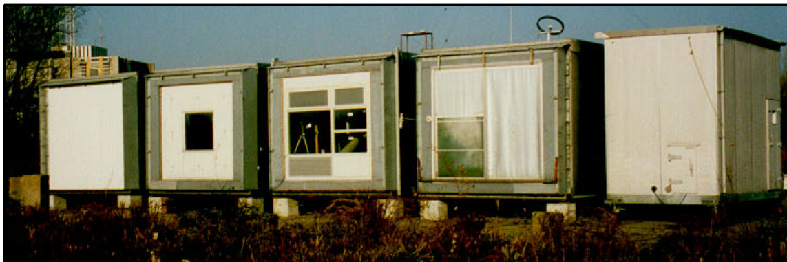
Figure 59: Photo of the TNO PASSYS test cells and moveable cold box (on the right)
